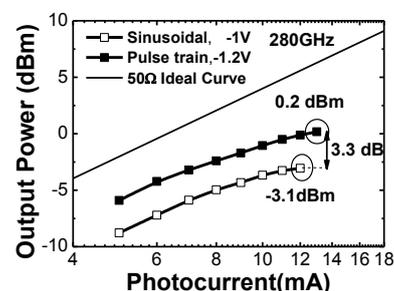
Figure 3. The measured photo-generated MMW power of NBUTC-PD (n-charge) with a 3  $\mu\text{m}$  active diameter of PD versus photocurrent under sinusoidal (open symbol) and pulse train (close symbol) excitations at 280 GHz operation frequency. Solid line is ideal trace for 100% modulation depth and 50  $\Omega$  load.
