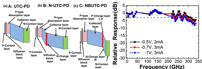
Figure 1. Conceptual band diagrams of (a) Device A: UTC-PD, (b) Device B: NBUTC-PD with n-charge and (c) Device C: NBUTC-PD with p-charge layers
