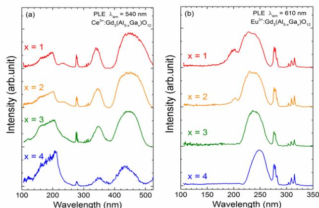
Fig.1. PLE spectra of (a)  $\text{Ce}^{3+}$  and (b)  $\text{Eu}^{3+}$  : GAGG.
