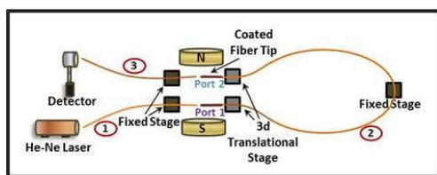
Fig. 1. Schematic of fiber-optic twin-cantilever set up
