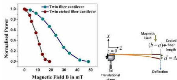
Fig. 2. Response of twin-fiber-cantilever configurations in external magnetic field (left) and schematic of bending of coated fiber (right)
