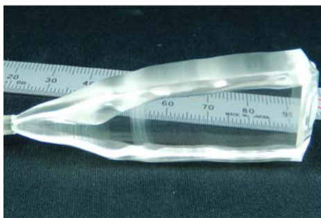
Fig. 1. Photograph of a CTGAS single crystal with x=2.25 .
