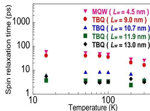
Fig.3 Temperature dependence of the spin relaxation time in narrow well.
