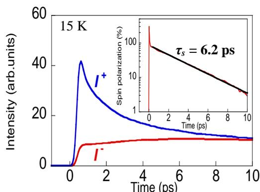
Fig.2 Time evolutions of cocircular ( $I^+$ ) and anticircular ( $I^-$ ) polarization at 15 K for the excitation power of 30 mW. The inset shows the time evolution of spin polarization.
