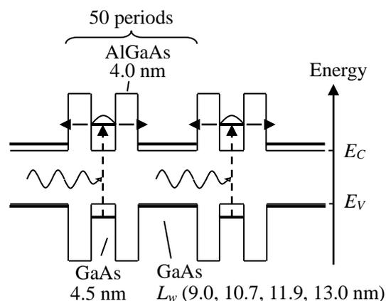
Fig.1 Energy band diagrams of the GaAs/AlGaAs tunneling bi-quantum-well.
