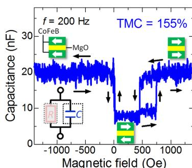
Fig. 2 TMC effect in MgO-based MTJs with a TMR ratio of 108%.
