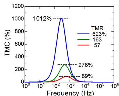
Fig. 3 Calculated results on the frequency dependence of TMC.
