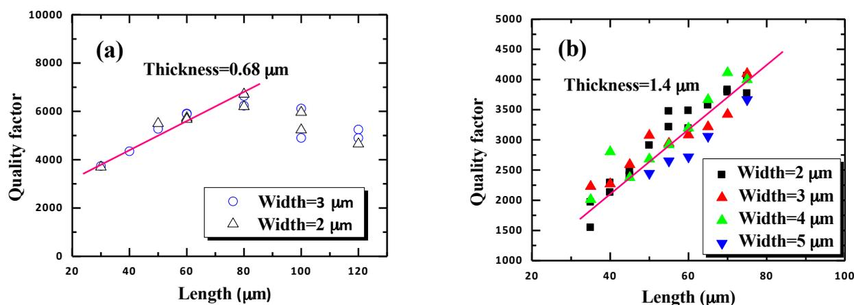
Fig. 1 Quality factor dependence of SCD cantilevers with different thicknesses (a) 0.68  $\mu\text{m}$  and (b) 1.4  $\mu\text{m}$
