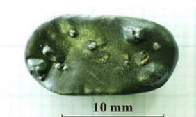
Fig. 1. View of the MW-synthesized bulk polycrystal for 60 mol% Ag<sub>2</sub>S.
