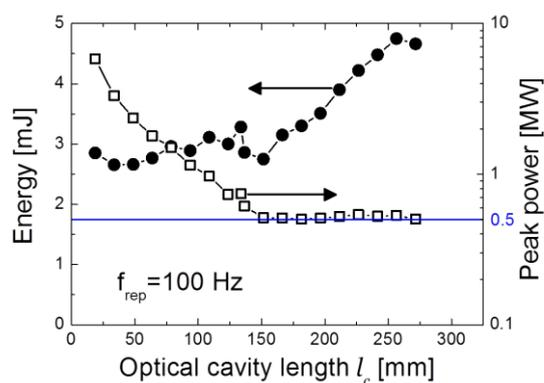
Fig. 2. Pulse energy and peak power versus optical cavity length.
