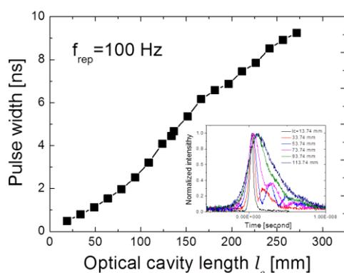
Fig. 1. Pulse width versus optical cavity length.
