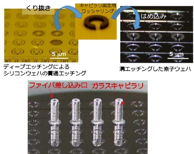
Fig. 2 Photographs of self-alignment process of glass capillaries to the detectors on Si wafer.
