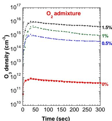
Figure 1: Temporal variation of O<sub>3</sub> density in DBD chamber.
