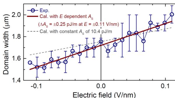
Fig. 1: Electric-field dependence of domain widths. Circles are obtained from experiments, and error bars are determined from five-region measurements. Calculated dependences are shown by solid line with electric-field dependent  $A_s$  as well as by dashed line with constant  $A_s$ .
