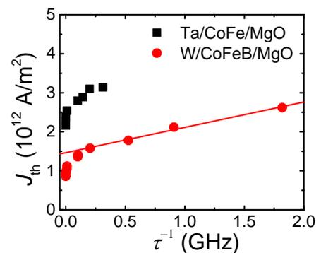
Fig. 1.  $\tau^{-1}$  dependence of  $J_{th}$  for W (Ta)/CoFeB/MgO structures.
