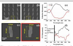
Fig. 1. (a-d) SEM images of the investigated plasmonic chiral nanostructures. (e) Dissymmetry spectra between left- and right-handed circularly polarized extinctions and (f) PLE induced by the chiral nanostructures.
