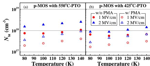
Fig. 2 Dependence of  $N_{bt}$  on  $T$  for p-MOS with (a) 550°C-PTO and (b) 425°C-PTO. The results with Al-PMA are also shown.
