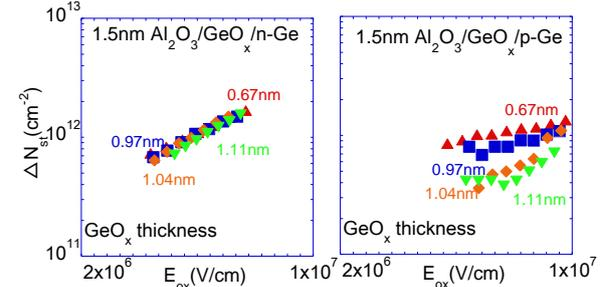
Fig.1:  $\Delta N_{st}$  of 1.5-nm-thick Al<sub>2</sub>O<sub>3</sub>/GeO<sub>x</sub>/Ge with plasma pre-oxidation time from 1 to 4s.
