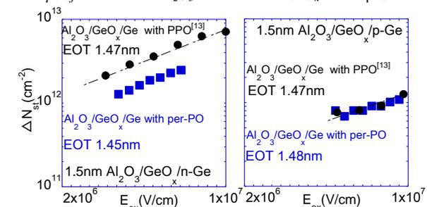
Fig.3:  $\Delta N_{st}$  of 1.5-nm-thick Al<sub>2</sub>O<sub>3</sub>/GeO<sub>x</sub>/Ge with plasma post or pre-oxidation with an EOT ~1.5-nm-thick
