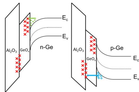
Fig.2: schematic diagram of possible position and origin of slow traps of 1.5-nm-thick Al<sub>2</sub>O<sub>3</sub>/1.04-nm-thick GeO<sub>x</sub>/n- and p-Ge
