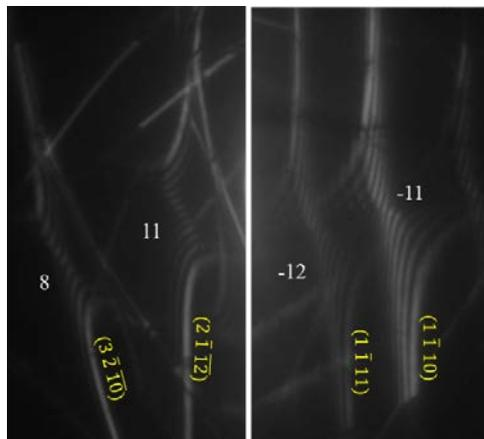
Figure 1: LACBED images at a  $\langle c + a \rangle$  TMD showing Kikuchi band splitting.
