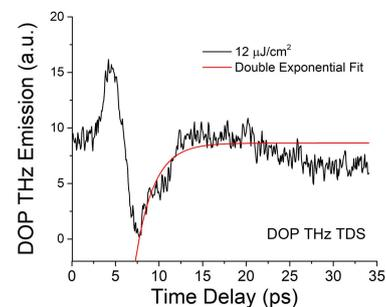
Fig. 2. Carrier lifetime evaluation through DOP THz-TDES at low carrier injection
