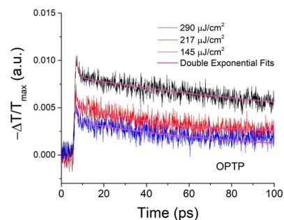
Fig. 1. Carrier lifetime evaluation through OPTP technique at high carrier injection levels
