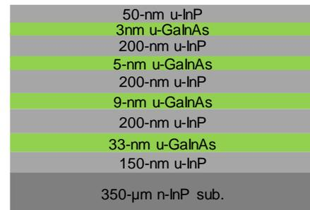
Fig.2. Wafer structure used for this investigation
