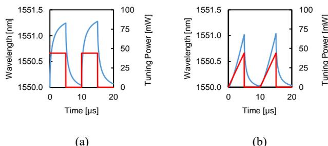
Fig. 2. The optical output signal (blue) for two different tuning signals (red), (a) rectangular signal, and (b) triangular signal.
