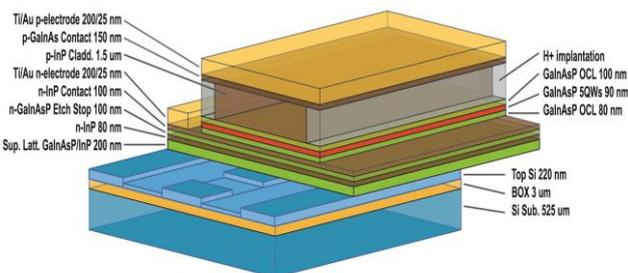
Fig. 1. Structure of GaInAsP/SOI hybrid DFB laser, tuning current is injected to the Si waveguide in the lateral direction.
