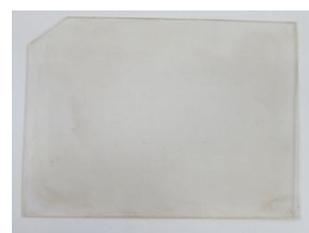
Fig.2 Photograph of transparent conducting film (5x6cm)
