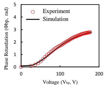
Fig. 2 The relationship between  $\Delta\phi$  and  $V$  of the PS-BPLC cell.
