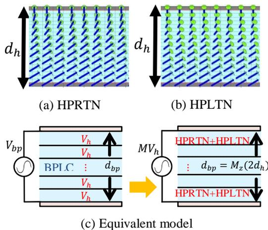
Fig. 1(a) An HPRTN cell. (b) An HPLTN cell. (c) an equivalent model for a BPLC cell.
