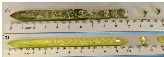
Fig2. TlBr crystals: (a) Purified material and (b) purchased TlBr powder.
