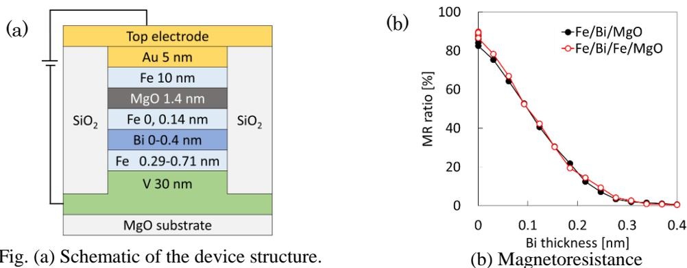
Fig. (a) Schematic of the device structure.
