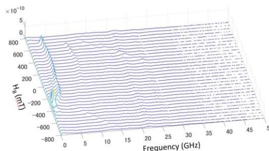
Fig. 2, Magnoise spectrum of a MTJ based STO as a function of  $H_B$ .
