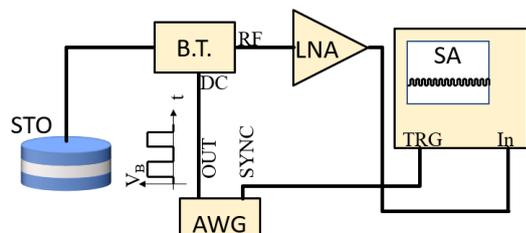
Fig. 1, Block diagram of high sensitivity magnoise measurement setup.
