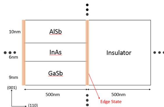
Fig1. Introducing insulator next to Quantum wall of InAs/GaSb
