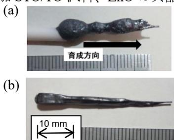
Fig.1. STO/TO eutectic materials grown by  $\mu$ -PD method. (a) undoped and (b) Nb-doped.
