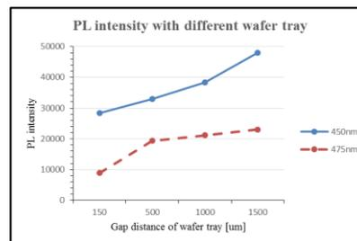
Fig.2 PL intensity dependence on wafer tray gap.
