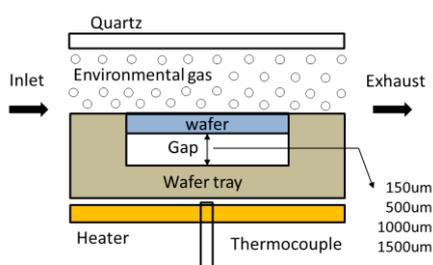
Fig.1 Schematic configuration of the MOVPE reactor.
