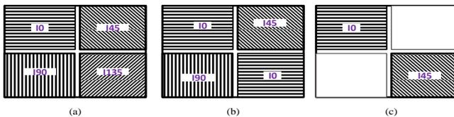
Fig. 1. Different MP patterns: (a) Equally weighted MP patterns with four different micro-polarizers; (b) Patterns with three micro-polarizers; (c) Patterns with two micro-polarizers.
