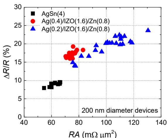
Fig. 1  $RA$ - $\Delta R/R$  of the CPP-GMG sensors with AgSn and Ag/IZO/Zn spacers
