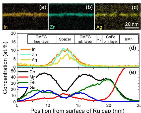
Fig. 2 EDS mapping and depth profile of the CPP-GMR film with Ag(0.4)/IZO(1.6)Zn(0.8) spacer.
