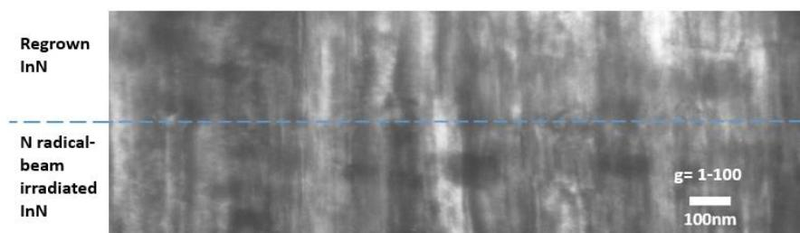
Fig. 1. Cross-sectional TEM image of the InN grown by ISRRI method with  $g = 1-100$ .
