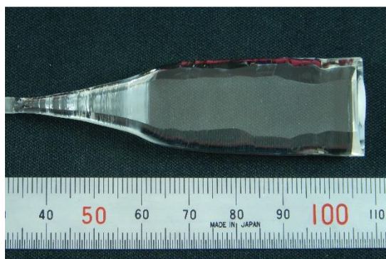
Fig. 1: Photograph of CTAS single crystal grown under \text{N}_2+1\%\text{O}_2 using a Pt crucible.
