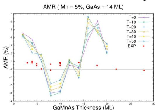
**Fig. 1.** The calculated film thickness  $d$  dependence and temperature dependence of the AMR in 14ML-GaAs /  $d$  ML-Ga<sub>0.95</sub>Mn<sub>0.05</sub>As SLs. The experimental data<sup>[2]</sup>(EXP) is measured at 5 K.
