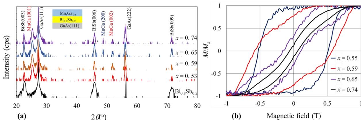
Fig. 1 (a) X-ray diffraction spectrum of several  $\text{Mn}_x\text{Ga}_{1-x}$  ( $0.53 \leq x \leq 0.74$ ) /  $\text{Bi}_{0.8}\text{Sb}_{0.2}$  bi-layers grown on GaAs(111) substrates (inset), and (b) their normalized magnetization hysteresis loops, measured by magnetic circular dichroism at room-temperature.
