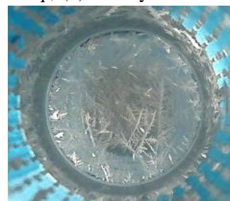
Fig. 1. Top view of the dendrite ice crystal observed under zero magnetic fields.
