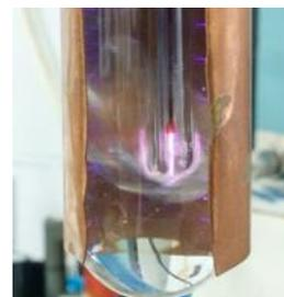
Fig. 2. Photograph of discharge in water
