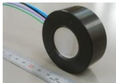
Fig. 3 CP gas detector for neutron imaging.
