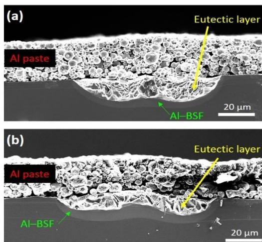
Fig. 1. SEM cross-sectional images of local Al contacts using (a) Paste A with no Si content in the Al paste, and (b) Paste B consisting of Si content.
