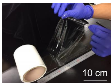
Fig. 1 PVA/PDMS bilayered film peeled off from PET substrate.
