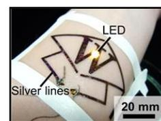
Fig. 3 An LED lighting circuit-laden SBS thin film attached to a skin surface.
