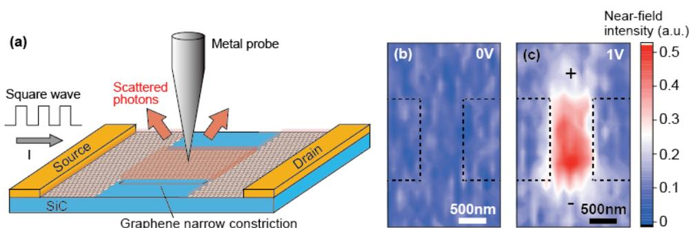
Fig. 1 (a) Schematic illustration of the experimental configuration used to detect current-driven evanescent wave on graphene narrow constriction device. The metallized AFM probe is used to scatter the near-field component to the THz confocal microscope. Near-field images were obtained with the bias of (b)  $0 \text{ mA}$  and (c)  $1.77 \text{ mA}$ , respectively.
