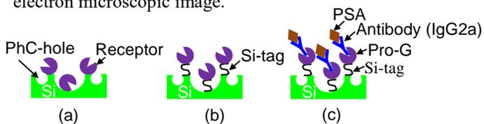
Fig. 2. Role of Si-tag (a) without Si-tag (b) with Si-tag and (c) role of Protein G.<sup>3)</sup>
