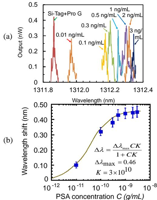
Fig. 3. (a) Experimental results of various PSA concentration and (b) Langmuir's fitting curve with experimental results.
