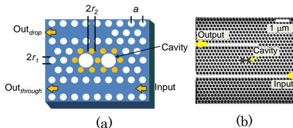
Fig. 1 (a) Schematic of proposed device and (b) scanning electron microscopic image.
