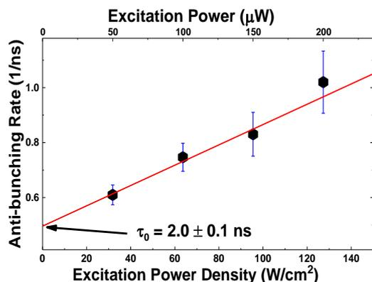
**Figure 2.** Power dependent decay rate of the confined exciton.
