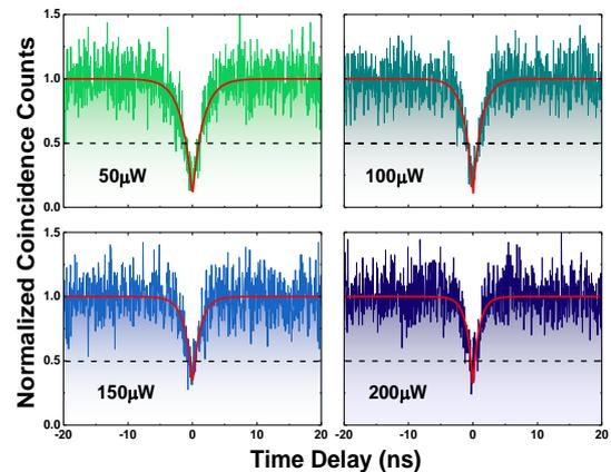
**Figure 1.** Power dependent autocorrelation measurements showing single photon emission.
