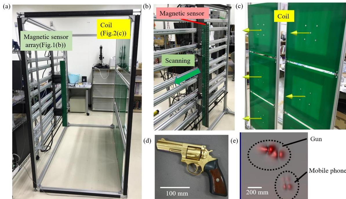
Fig.1 (a)Security inspection system., (b)Magnetic sensor array., (c)Coil., (d)Gun for the testing., (e)Reconstructed image obtained by security inspection system in Fig.1(a).
