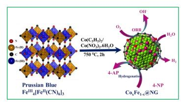
Schematic illustration for the synthesis of MOF derived nanoalloy encapsulated in N-dope graphene layers.
