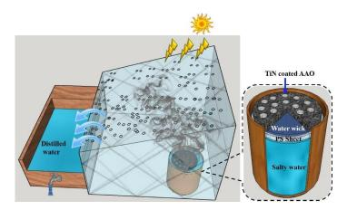
**Figure:** Schematic shows Titanium nitride (TiN) coated anodized aluminum oxide (AAO) converts the incident solar energy into thermal energy by the photothermal conversion and generate steam efficiently.
