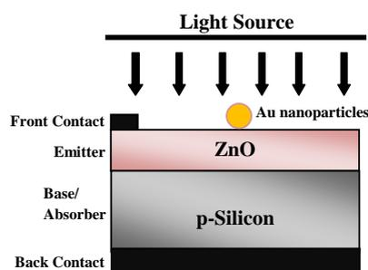
Figure 1: Schematic diagram of ZnO/p-Si solar cell with gold MNPs on top of ZnO layer.
