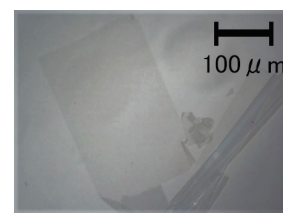
FIG 1. An optical microscope image of the thin sheet transferred on a glass plate.
