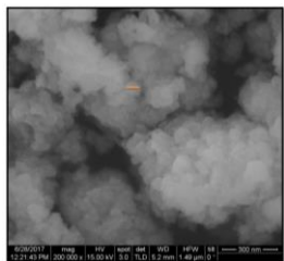
Figure 1 SnS nanoclusters of size \sim 100 nm
