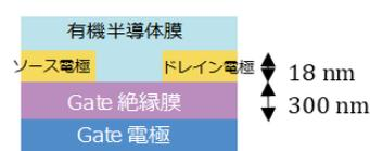
Fig.1 : Schematic of bottom-contact bottom-gate OTFT.
